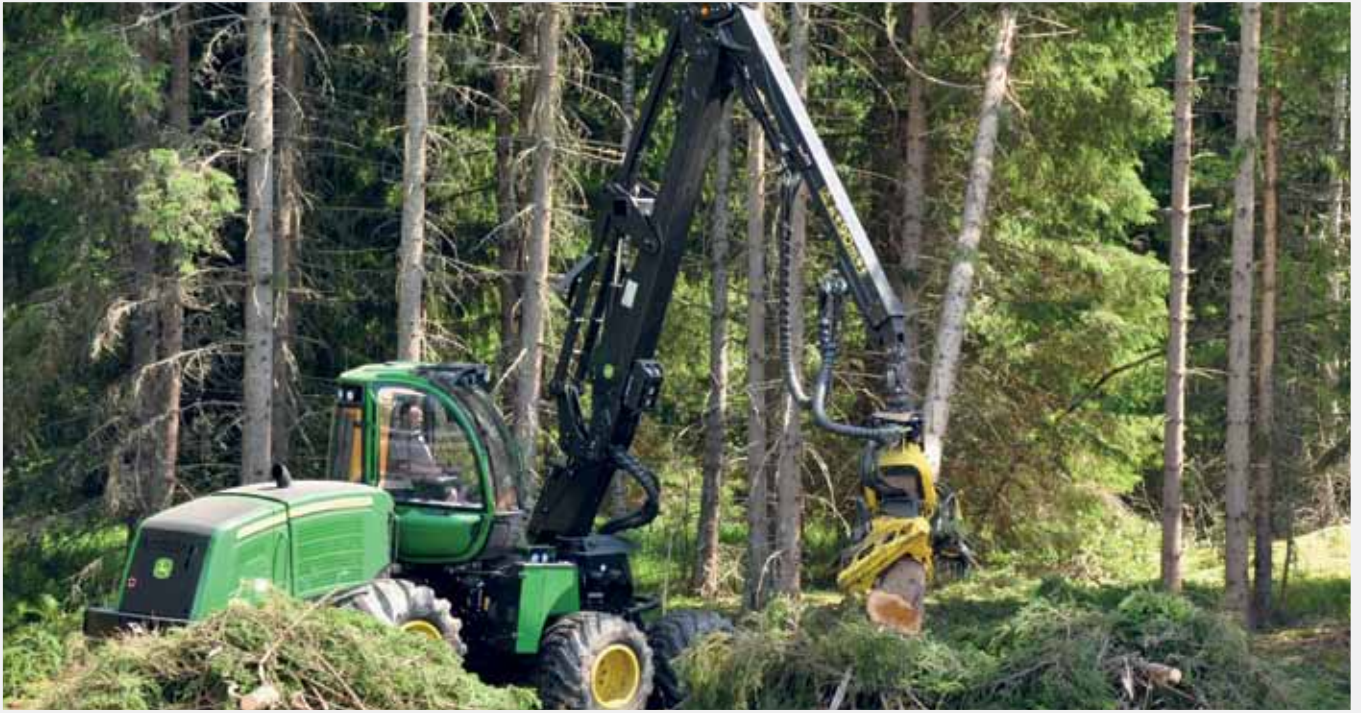
Integration with traditional logging is a prerequisite for cost efficient procurement of forest fuels. Almost half the round-wood produced by the harvester will end up as secondary fuel (bark, liqueurs, etc.) as it is processed in the industry. The harvester also prepares logging residues in tidy heaps for subsequent forwarding, storing and chipping. Photo: Rolf Björheden.
